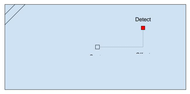
The camera units have two components: the camera and its attached microcontroller. The microcontroller will receive the input from the cameras. From the input, a simple color detection routine will scan the frame for high blooms of light. Once a bloom is detected, the screen space positional coordinates of the bloom will be sent to the central server.
