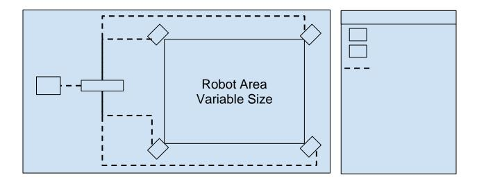
The above illustration elucidates the general hardware setup for the tracking system. In addition to the physical configuration, the software will need to be configured. In the central server, each individual camera's position and orientation must be recorded with exact precision. More than four cameras can be setup to increase accuracy and reduce tracking dead zones, but a larger ethernet switch may be required.
